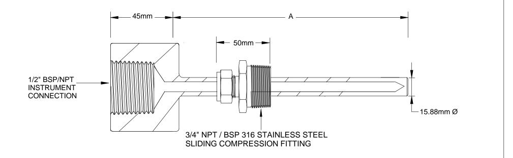
316 STAINLESS STEEL BARSTOCK PARALLEL THERMOWELL WITH COMPRESSION FITTING
